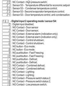
: NC Contact - Low pressure switch; : Sensor S4 - Insufflation temperature (indication). Note 1: When the digital input is configured as a pressure switch contact, it allows turning off the compressor, fan and defrost outputs, displayng the alarm associated with the source input. When the pressure switch event clears, the controller returns to the configured initial process.
