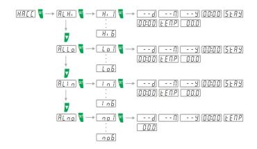
Note 2: The alarm duration time and the maximum measured temperature can be updated while the alarm is ocurring
