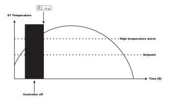
Up to 6 records of each alarm type are stored. If the number of stored records exceeds this amount, with each new alarm, the least recent record is replaced.
