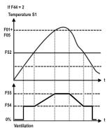
Note: If economizer mode is activated, functions F01 and F05 will be replaced by F02 and F06, respectively.
